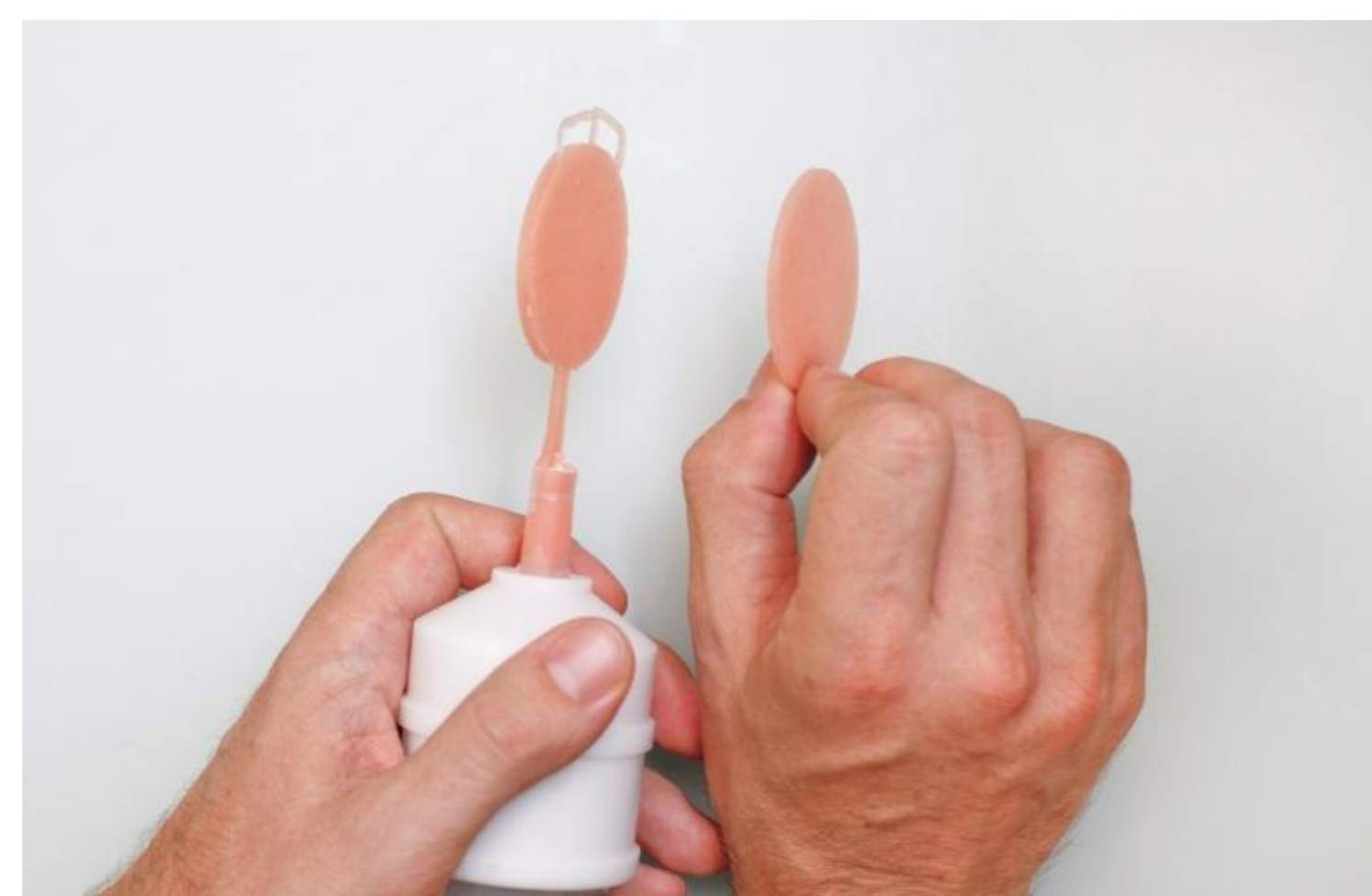
Left: polymerized ingot; right: ground ingot
