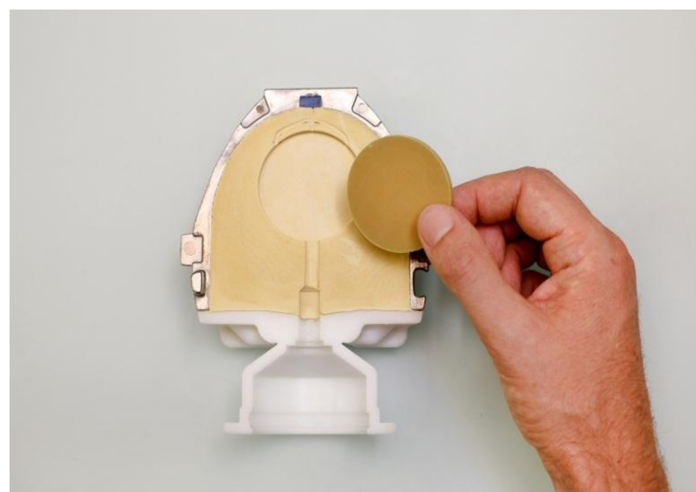
Investment of the silicone spacer to produce the ingot for residual monomer measurement
