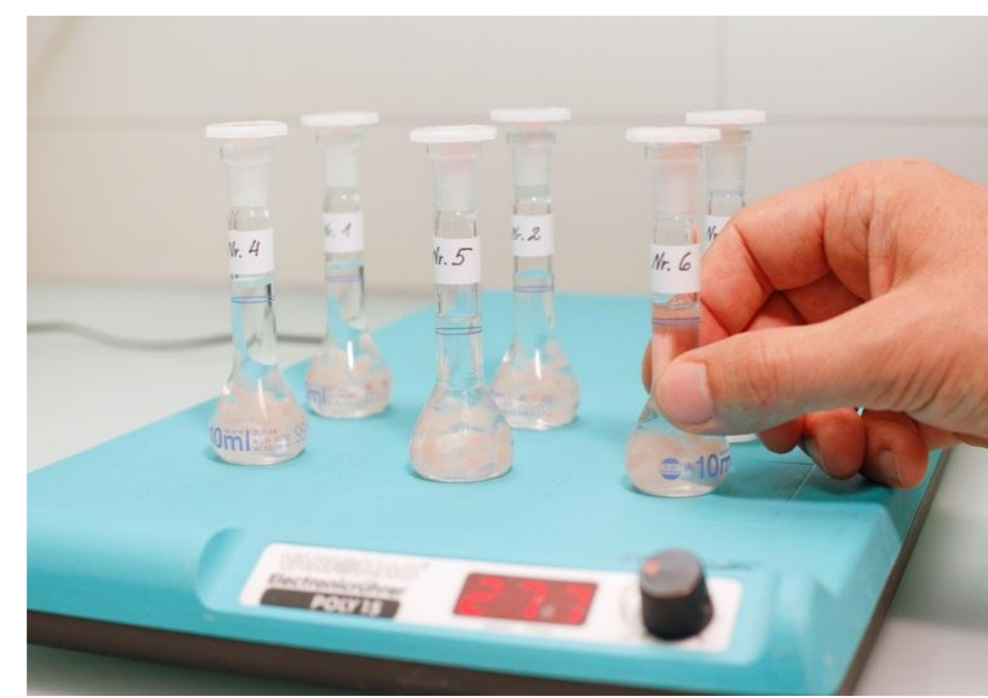
Extraction of methyl methacrylate by stirring in acetone for 72 hours
