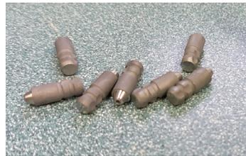
6. Unscrew the prosthetic from the master cast. Attach the roughened scan analogs to the prosthetic.
