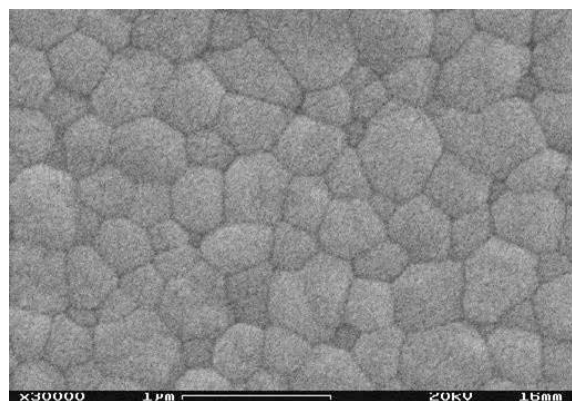
Fig. 5: Sintering structure of IPS e.max ZirCAD (SEM, thermally etched at 1420 °C for 15 min.)
